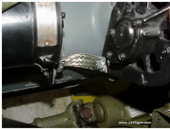
FM-GPW-18857 Bond Strap, this strap is connected to the generator base to the starter base
