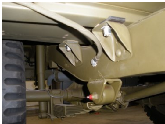
FM-GPW-14513 Bond Strap, this elusive cable is found under the tub and connects to the radio terminal box.
